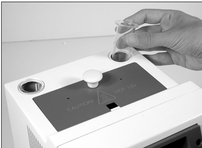
Figure 3. Mounting the glass Capillary Holders.
